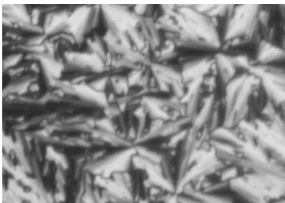
FIGURE 5 Optical texture characteristic of the pyrazine-bridged dirhodium carboxylates in the hexagonal mesophase.
